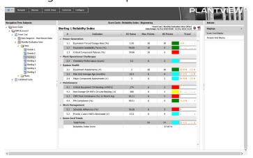
The Analysis Grid View offers a condensed view of Reliability Index information within a single cell. The displayed value and background color of a grid cell is configurable. For items implementing the same Score Card Template, adhoc versions of several views are provided to facilitate comparing Reliability Index performance between different selections that would not be possible with the standard hierarchy of equipment/facilities.
